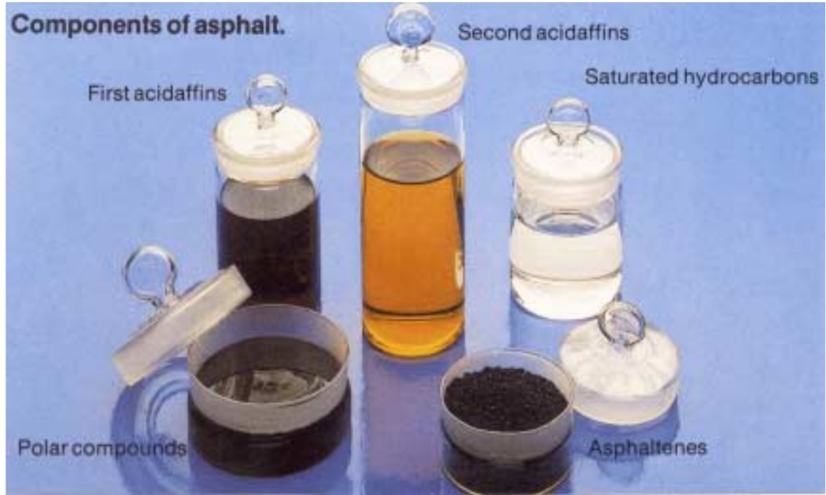
Figure 1. Asphalt Binder Fractions, Asphaltenes and Maltenes.
